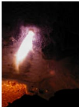
Typical PYROX™ flame in Electric Arc Furnace
