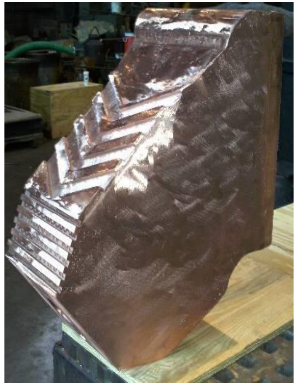
Water-Cooled Copper Panel
